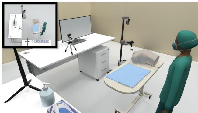
Fig. 1. Artificial rendering of the training environment and ASTRID, which is composed of the Stretch robot, a depth camera, and a computer screen.
