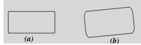
Figure 5: (a) is a rectangular part. (b) shows a box to contain the part with all possible orientations when the uncertainty \phi = 0.1 .
