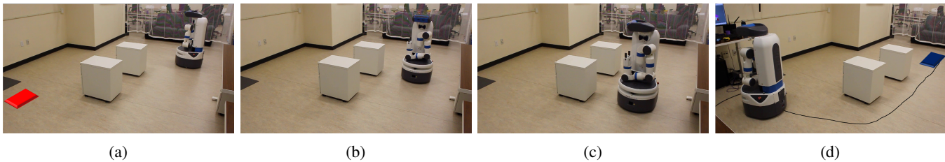
Fig. 11: Physical validation of OPCPS with caching for the lab domain. The Fetch requires to reach the table in (d) while avoiding white cabinets. The red rectangle in (a) and the blue rectangle in (d) represent the target and the start locations, respectively. The black line is the traversed path while following the policy generated by OPCPS with caching.
